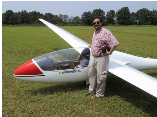
Fig 4. The Standard Cirrus, 15-m wingspan, single seat, all composite test sailplane
