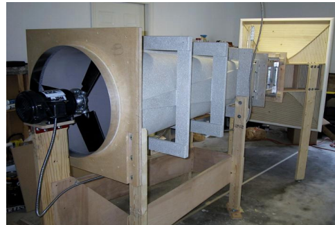
Fig.7. SINHATECH Low-Speed Wind Tunnel
