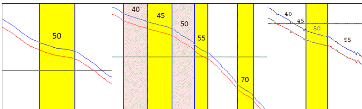
Figure 3– Repeated Abrupt Changes in Sink Rate at Start and End of High Performance Speed Runs
