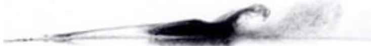
Figure 1: Smoke Image of Transition from Laminar to Turbulent Flow (Greg Cole and Prof. Mueller, Notre Dame)
