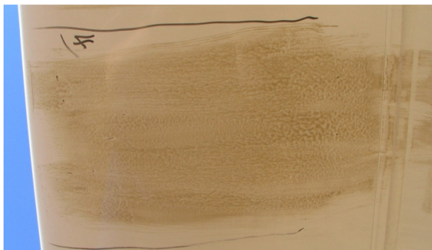
Figure 14: Modified Lower Surface Oil-Flow Image
