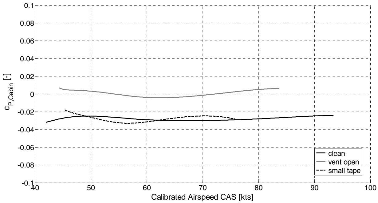
Figure 12: Coefficient of corrected cabin pressure vs. Calibrated Airspeed
