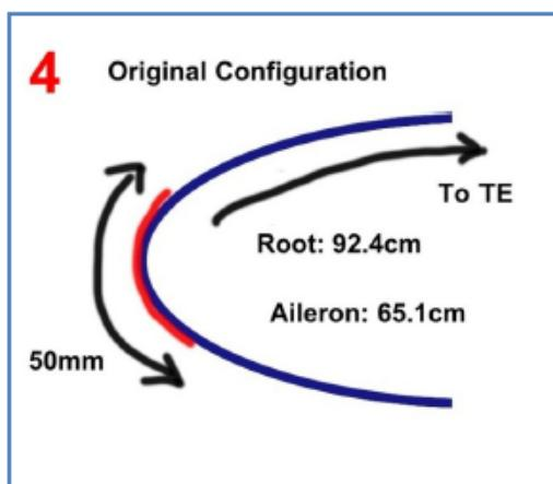
Figure 4: Position of „wide tape“ on inner wing leading edge according [4]
