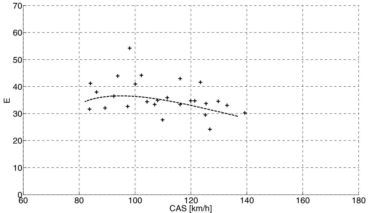
Figure 24: Configuration „small tape“, Comparison flight results (line) vs. partial glide analysis (symbols)
