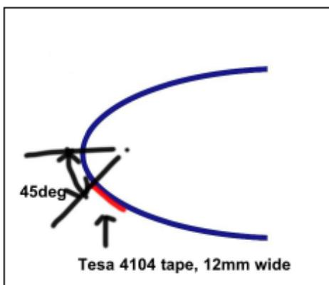
Figure 2: Position of „small tape“ according [4]
