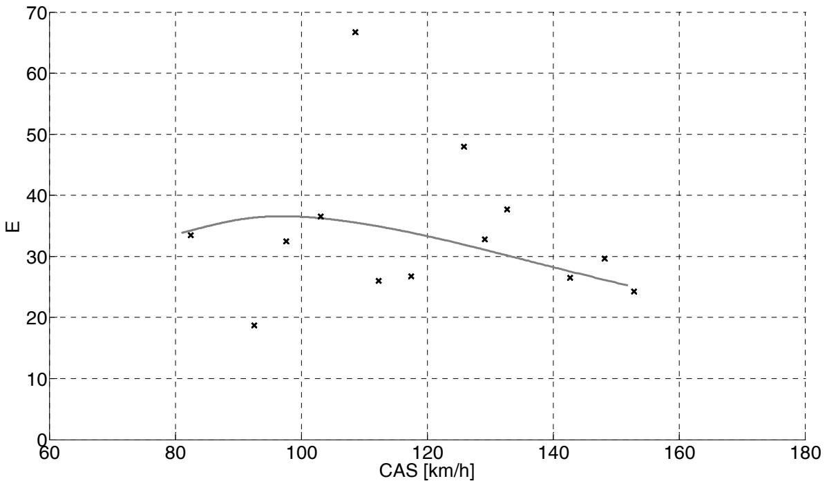
Figure 23: Configuration „vent open“, Comparison flight results (line) vs. partial glide analysis (symbols)
