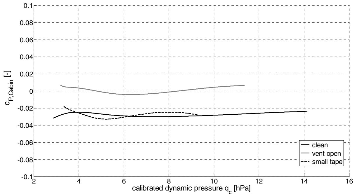
Figure 13: Coefficient of corrected cabin pressure vs. dynamic pressure
