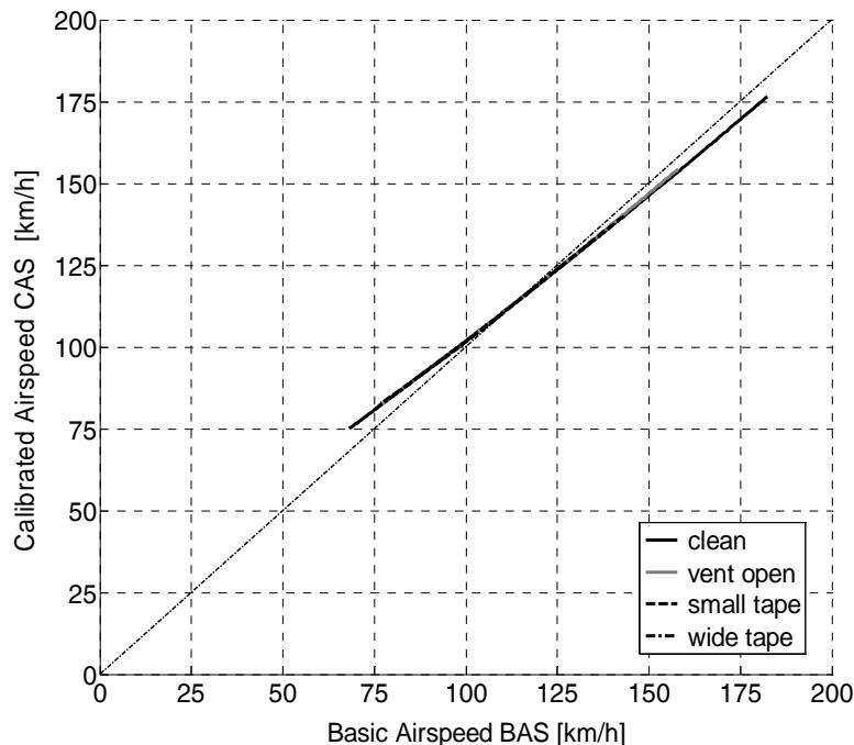
Figure 14: Airspeed calibration, CAS-BAS-depiction
