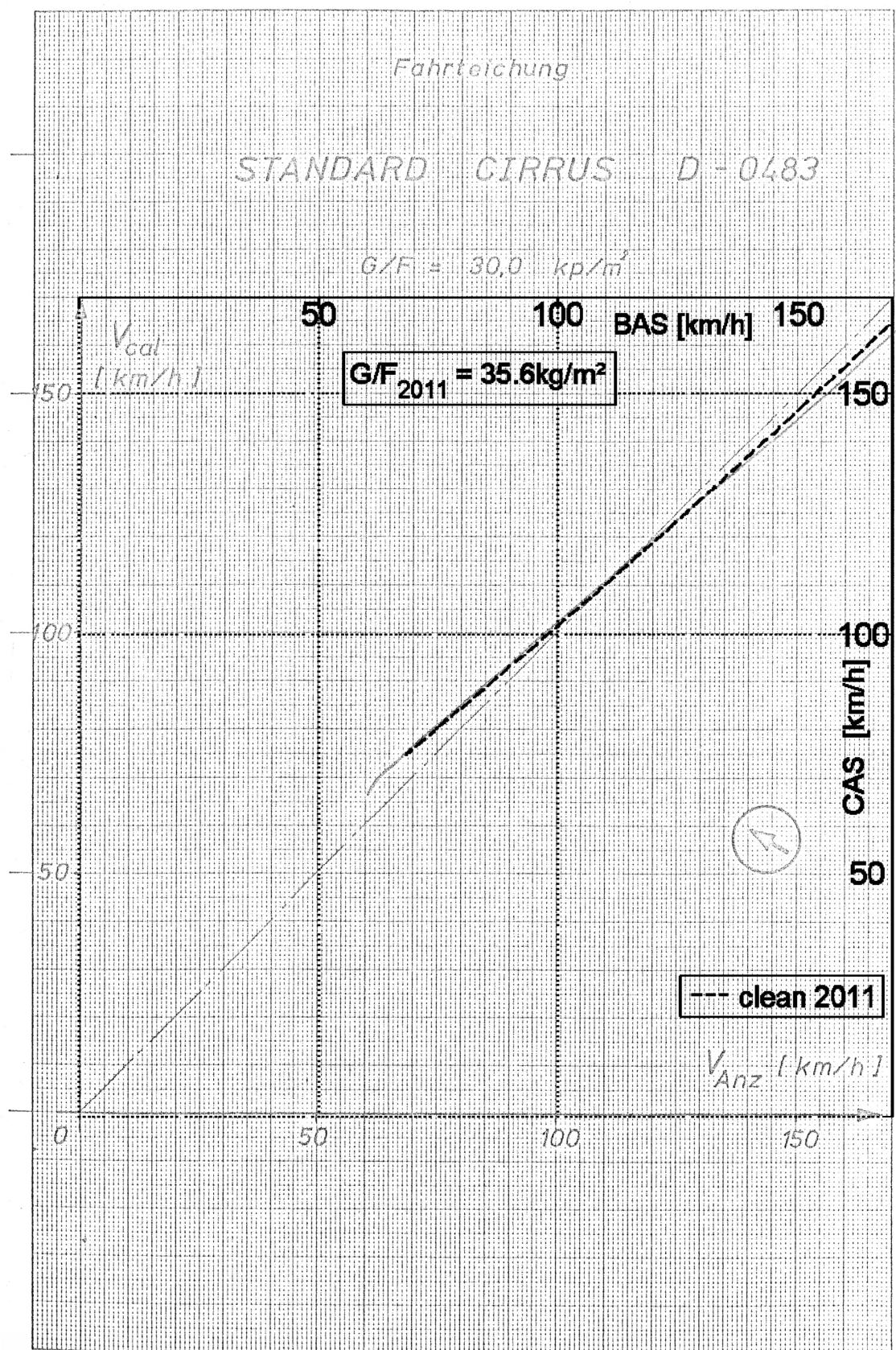
Figure 15: Comparison of airspeed calibration in 1971/72 [7] and 2011
