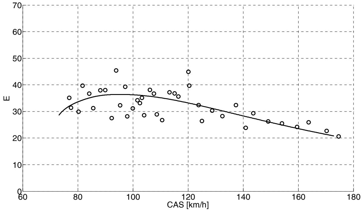
Figure 22: Configuration „clean“, Comparison flight results (line) vs. partial glide analysis (symbols)
