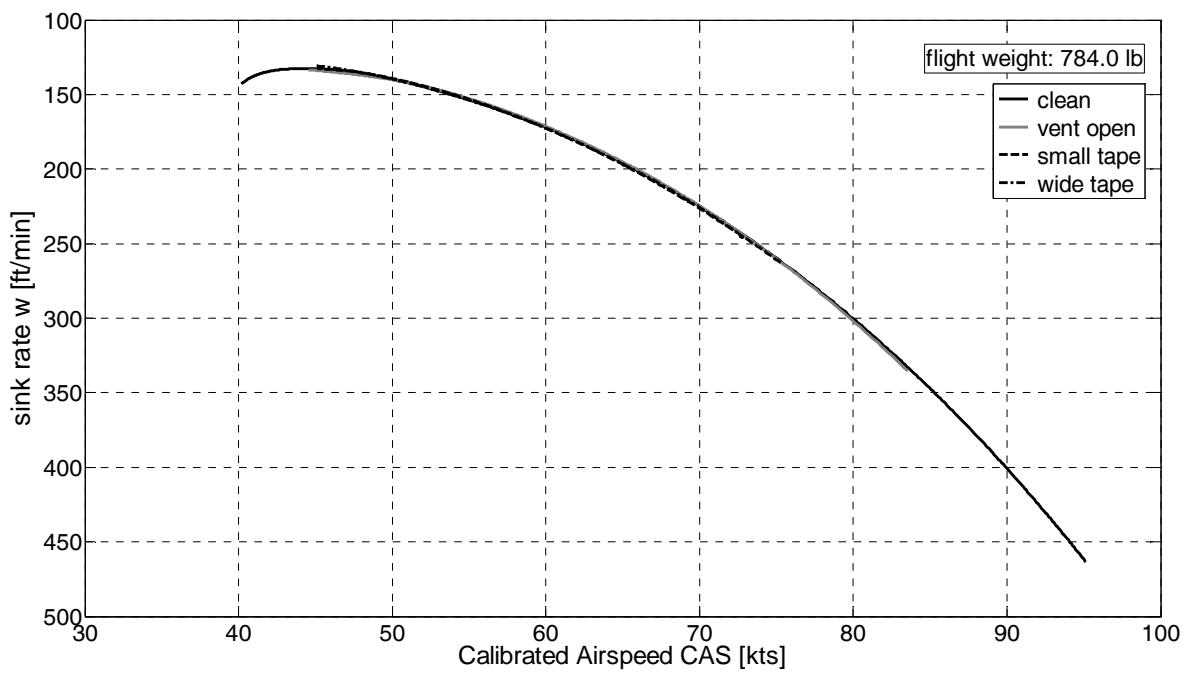
Figure 7: Sink rate vs. Calibrated Airspeed at reference weight
