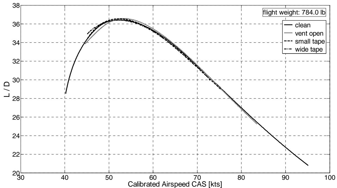
Figure 8: L/D vs. Calibrated Airspeed at reference weight
