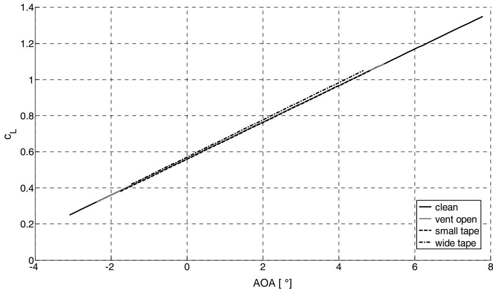
Figure 11:  $c_L$ -AOA-diagram
