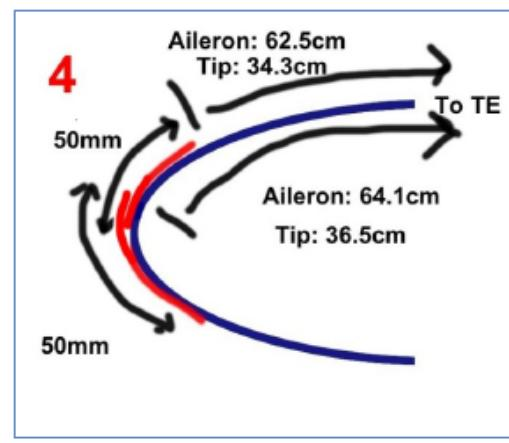
Figure 5: Position of „wide tape“ on outboard wing leading edge according [4]
