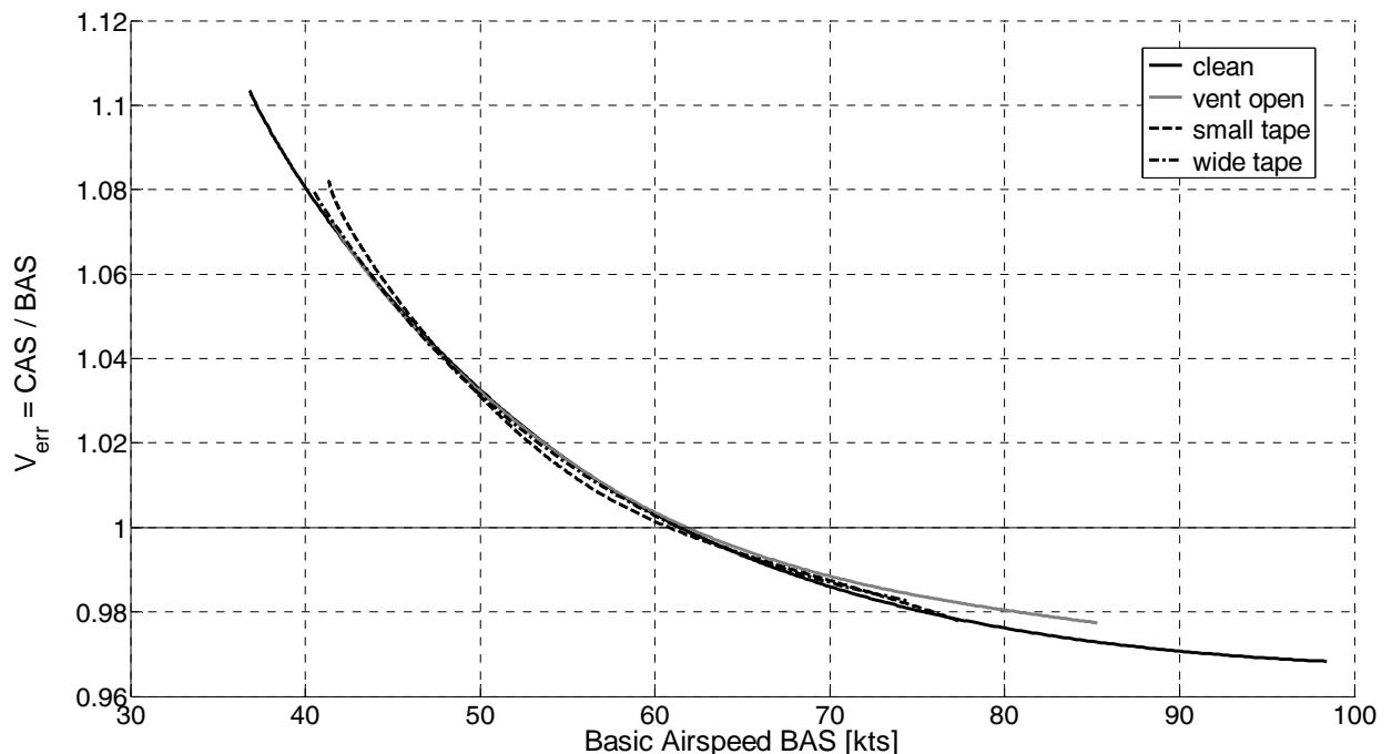
Figure 6: Airspeed calibration, CAS/BAS-BAS-depiction
