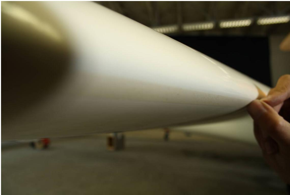
Figure 3: „small tape“ on right wing leading edge
